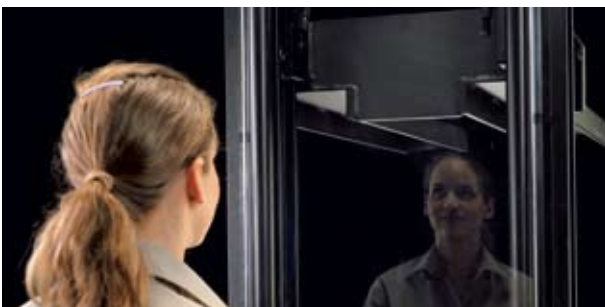
The BT Totalview design concept ensures the fork tips are visible from the operating position
