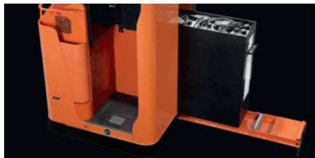
The battery on S-series models is seated on rollers with a built in battery table, allowing easy sideways battery exchange
